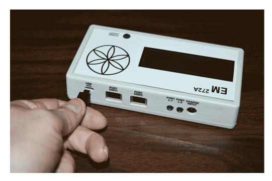
For the EM272A, make sure the unit is OFF and plug the Mini-USB cable into the mini-USB jack. The EM272A is OFF if the green LED ring light is not lit.
