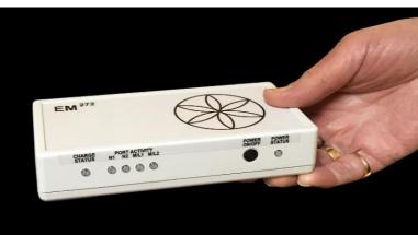
On the EM272, there are 5 lights on the left. The first one is the Charge status, (Green when fully charged; amber/red when low charge). The second and third lights show that the Nasal Probes (L and R) are attached. They glow green when in use. Lights four and five show that the Magnetic Discs (L & R) are attached. They also glow green when in use. On the Right is the Power button-
